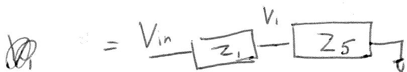
$$V_1 = V_{in} \frac{Z_5}{Z_1 + Z_5}$$
