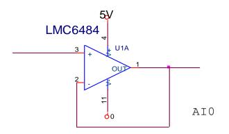
This year we will often use a quad op-amp which has 4 op-amps on a single 14 pin chip. See the data sheet linked on the course website for the pin diagram. We will be using the LMC6484. This op-amp can run on the 0 to 5V power supply from the USB. Here is an example of a built circuit, please don't try to trace the wires out, build yours from the schematics. In the photo below, some wires are neatly tucked away under the connector where you can't see them.
