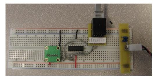
Once you insert the op-amp buffer between the sensor and the data acquisition system, you should get an accurate reading for the acceleration using the sensitivity from the sensor's data sheet. You need one buffer for each of the 3 acceleration components.
