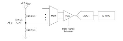
The 32 K resistor on the output of the chip and the resistor network on the input to the DAQ are interfering with each other. On the accelerometer diagram, the voltage at the "output amp" is the accelerometer voltage that we want. An analysis of the circuits connected to each other would show that there is a voltage drop across the 32 K resistor and thus an error in the acceleration measurement.
