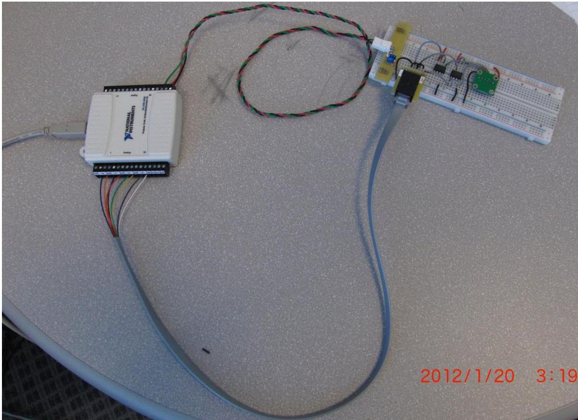
Here is a close up of the breadboard connector for the data. The pins go straight to the breadboard and the label tells you the color of the wire that the pin is connected to. You will run a wire from your circuit to this connector in order to measure the voltage.
