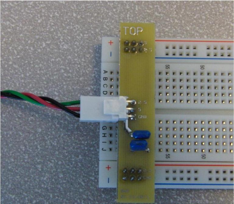
On the DAQ, the black, green, and red wires are connected to Ground, +2.5V and +5 V. Again it is common for these wires to shear off, so it is good to check the quality of the connection before starting.
